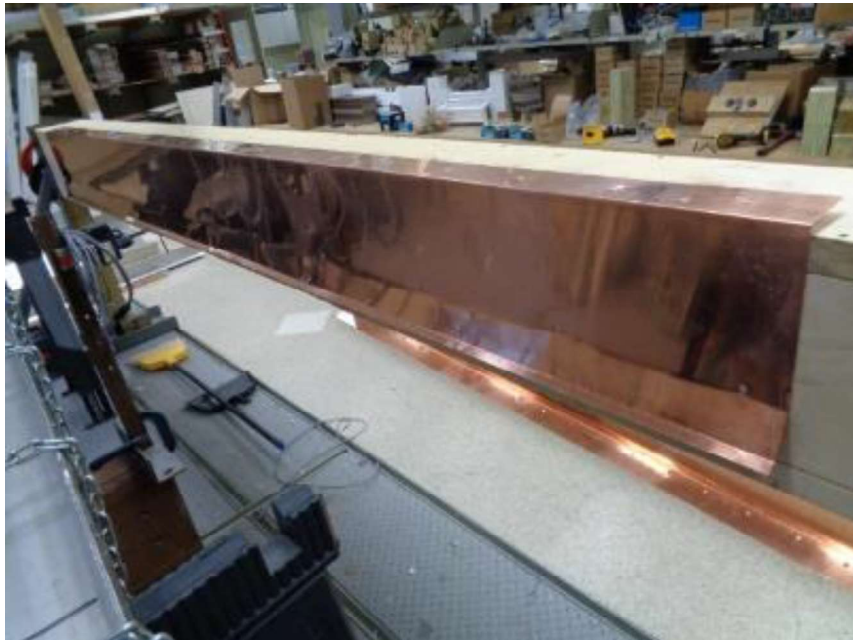
Photo No. 4 ANSI/SPRI Test RE-2, Failure of Copper Cleat, Bent to Release Fascia
