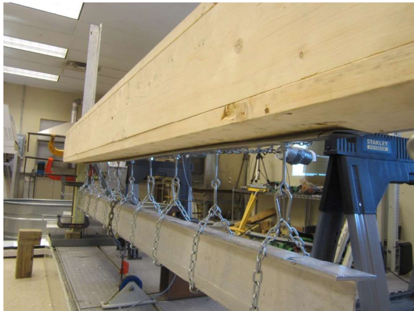
Photo No. 6 ANSI/SPRI Test RE-3, Coping Pull-Off Test In Progress Face Loading Shown under Load
