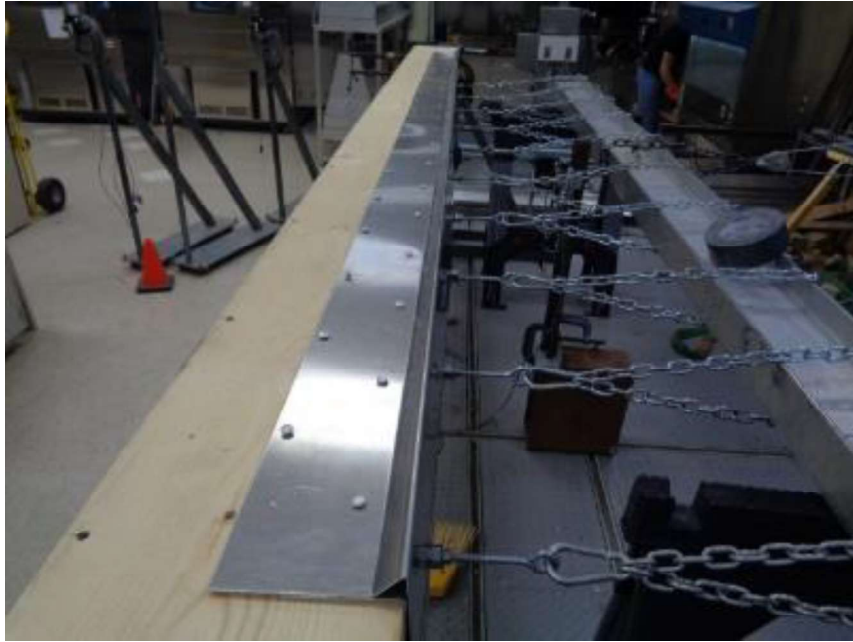
Photo No. 3 ANSI/SPRI Test RE-2, Test Setup
