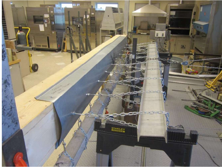
Photo No. 5 ANSI/SPRI Test RE-3, Coping Pull-Off Test In Progress; Tested with Face Down
