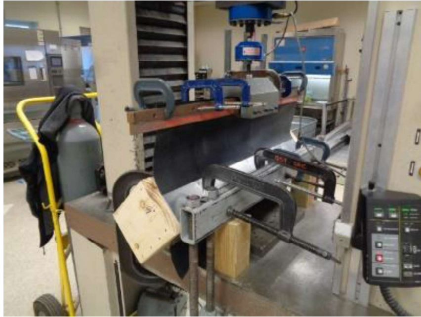
Photo No. 1 ANSI/SPRI Test RE-1 Test Set-up
