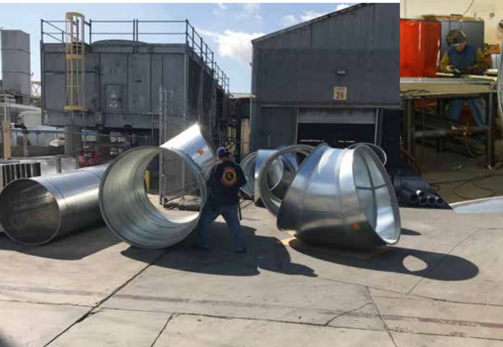
FROM LEFT TO RIGHT: A look inside of an autoclave at Boeing's Wing Center; 60" spiral ductwork will be installed high overhead; 48" saddle installed on 72" spiral trunk; 84" round x 14 gauge welded transitional fitting.
